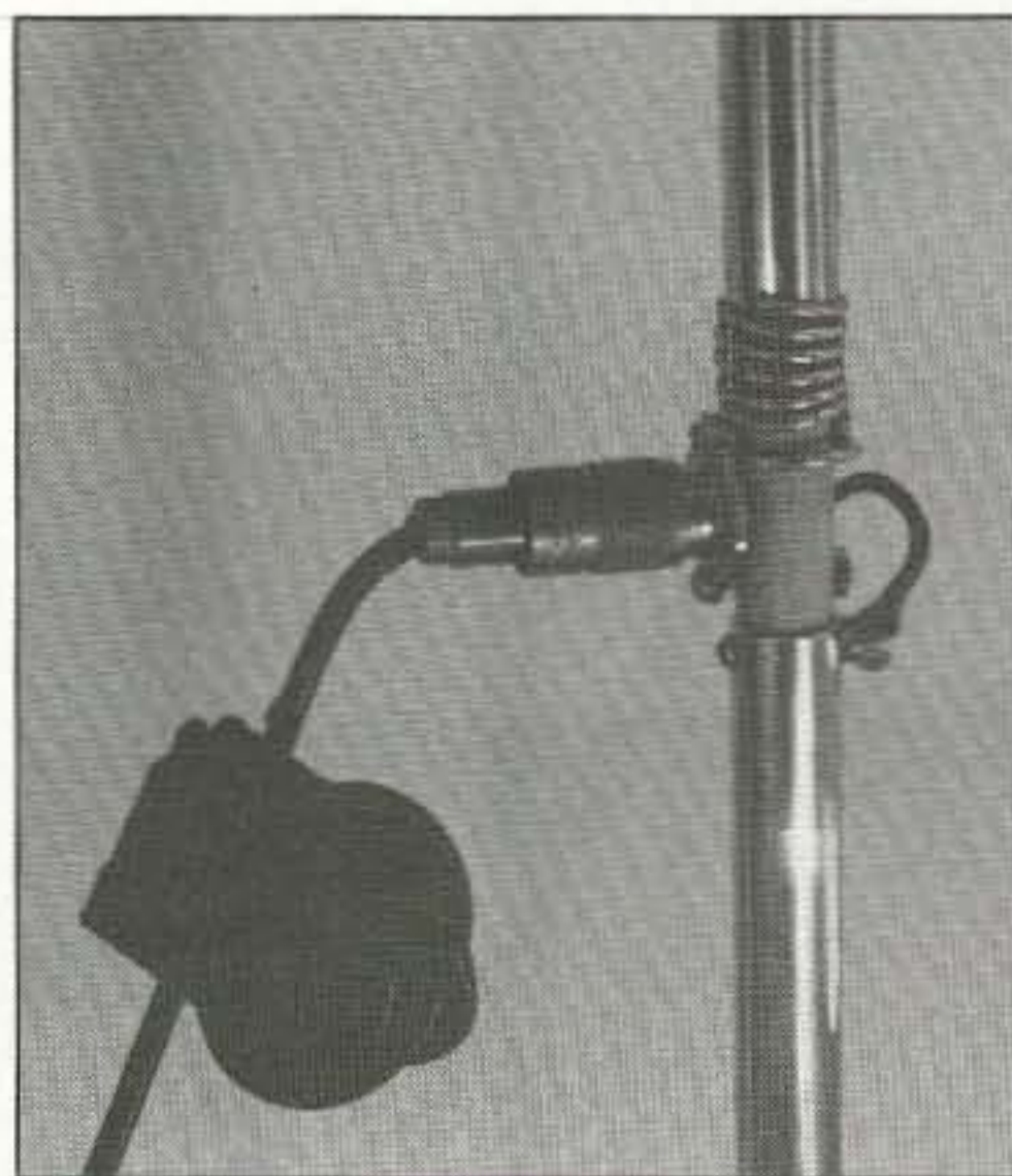
Photo D. The spring-loaded center insulator. Use a current balun (RF choke) at each end of the coaxial cable. The one shown has 5 turns of RG-58 coax wound on ferrite cores (Radio Shack 273-104).
