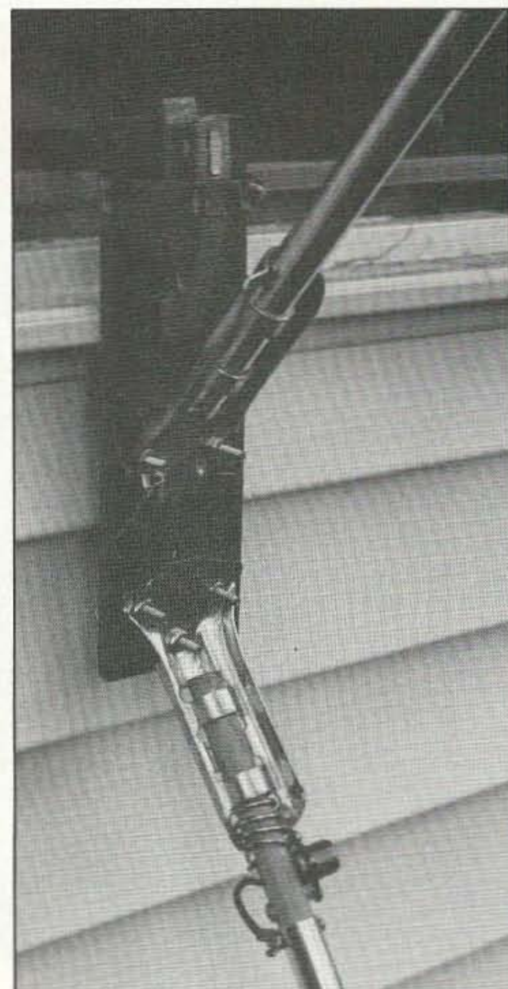
Photo G. A closer view of the window mount in operation. Notice that the indoor dipole's coax connector and center insulator are used here also. The compression spring fits into the mounting bracket and is the electrical connector to one element of the dipole.
