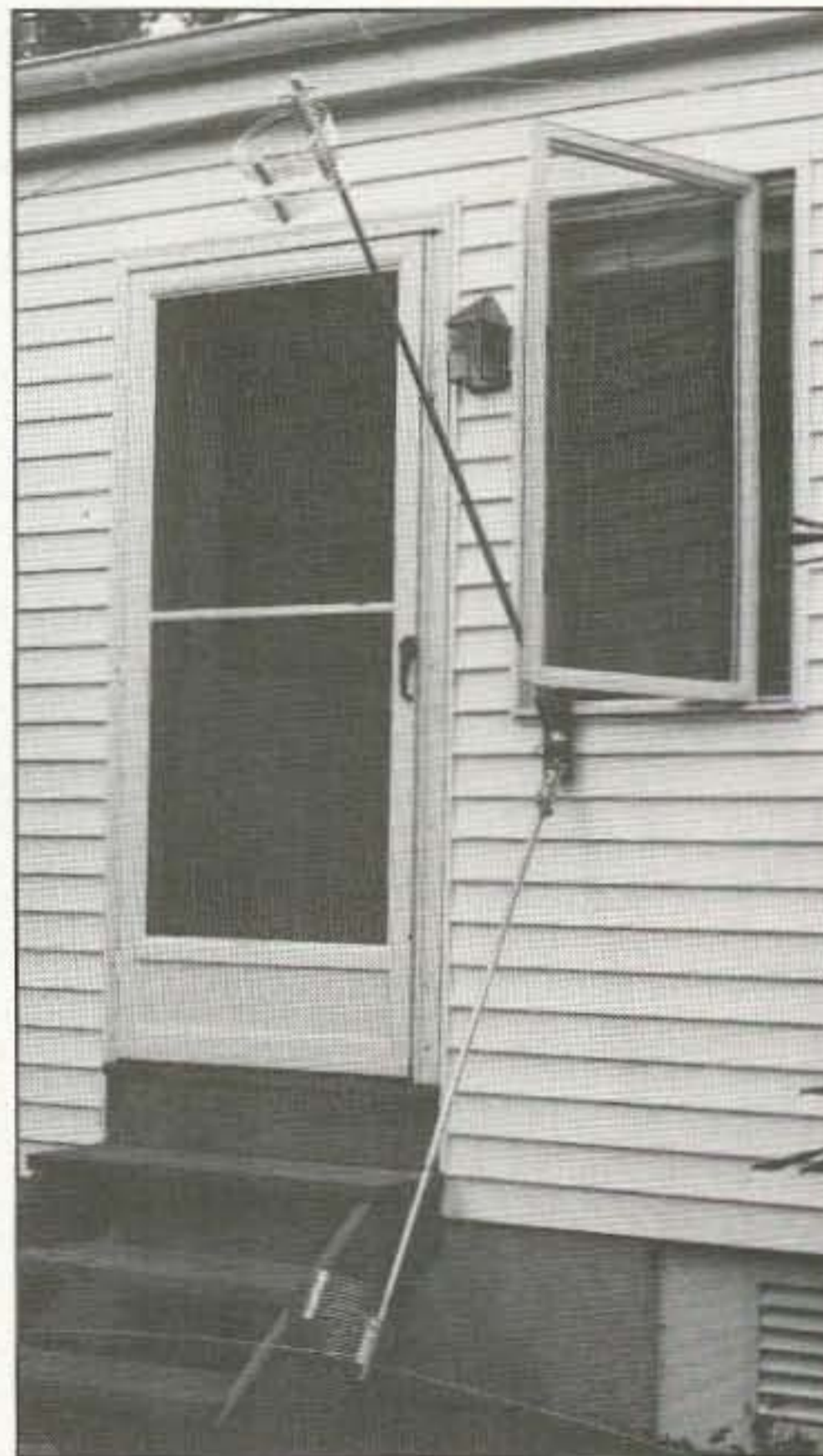
Photo E. The indoor vertical dipole can be window-mounted for better performance. A first-floor window was used for the photo, but the antenna should be as high and clear as possible. Extra coils with 5 turns (top) and 10 turns (bottom) may be added to the antenna, as shown here, for operation on 30 and 40 meters.
